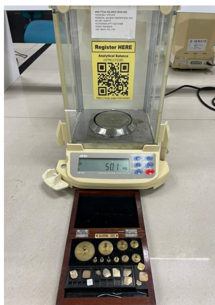
Figure 21. Semi-micro balance calibrated prior to usage
