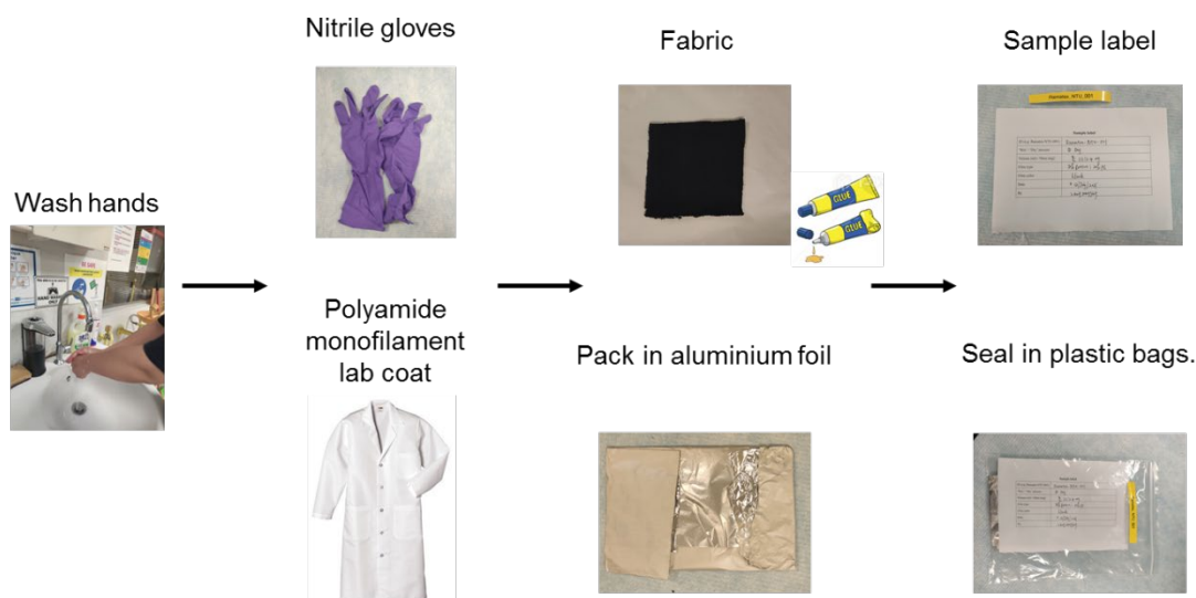
Figure 2. Schematic of experimental design for packaging the dry sample
