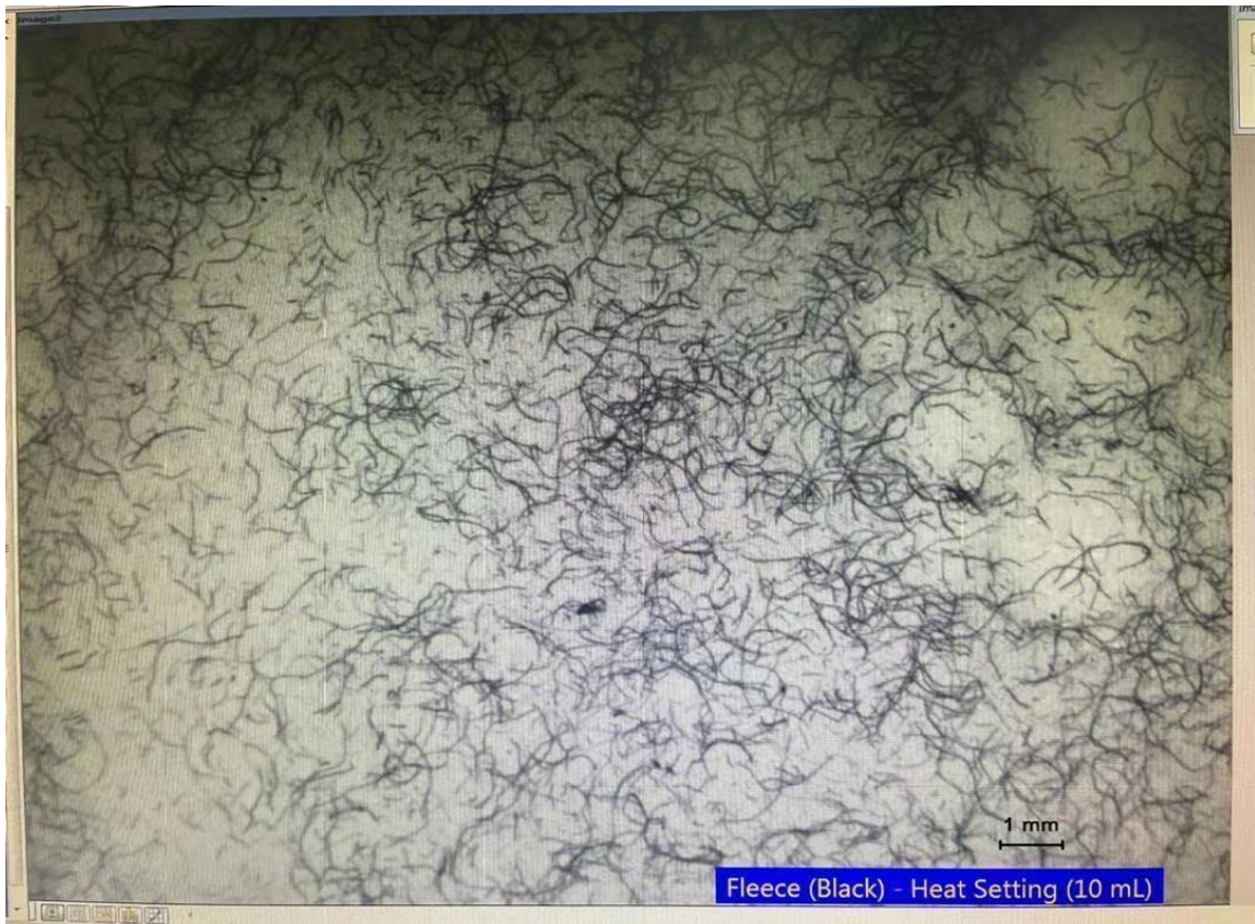
Figure 29. Fragments from analysis of 10 mL water from Fleece (Black) – heat setting process
