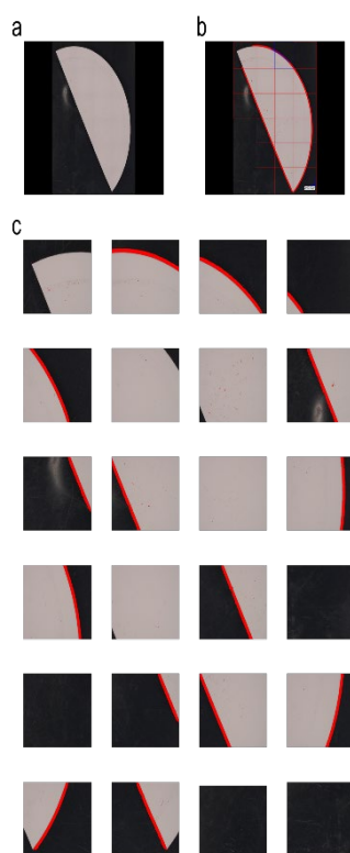
Figure 10. a Snapshot of a filter image for textiles, b A large composite image digitally stitched together from multiple snapshots, and c Individual images of the filter by the KEYENCE microscope.
