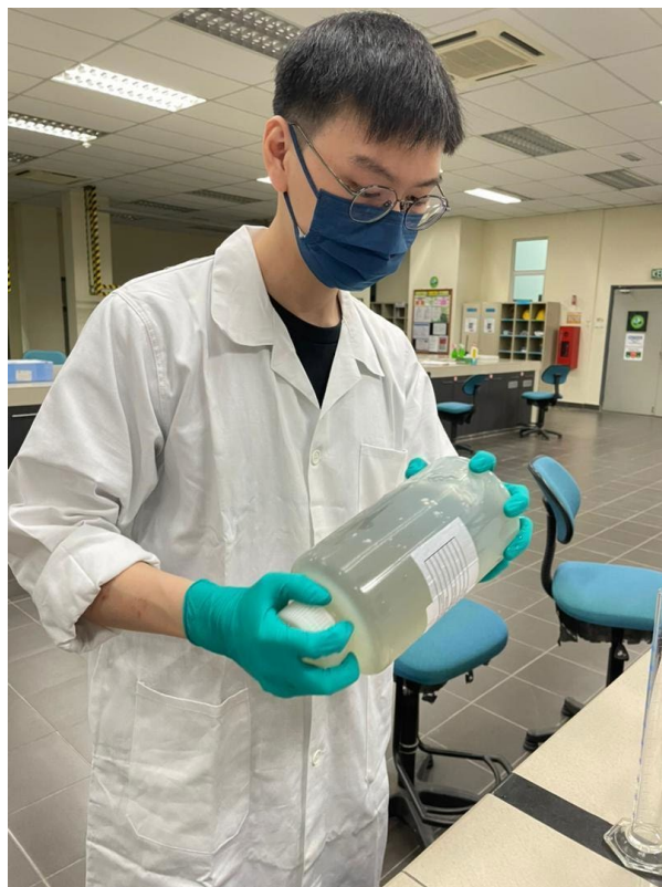
Figure 23. Samples are mixed vigorously before filtration
