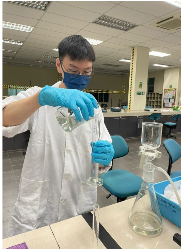
Figure 24. Desired sample volume is being measured using graduated cylinder
