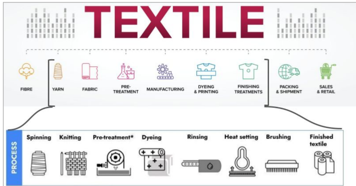
Image 2: General process of textile manufacturing
