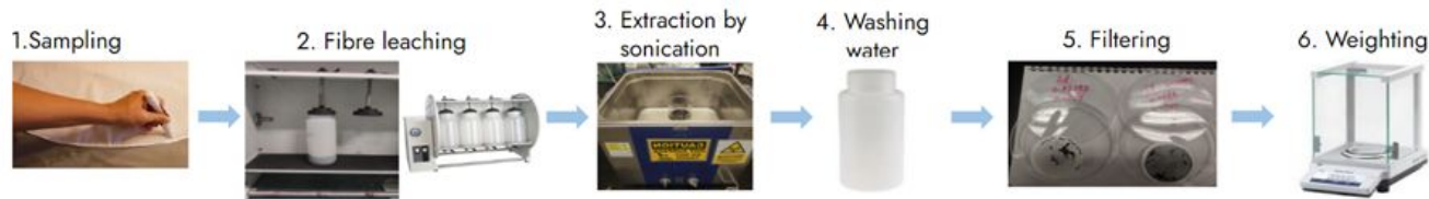
*Image 15: Flowchart illustrating the microfibre reattachment test
